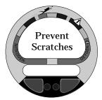
If the transparent face becomes scratched, Aeris can replace it, although small scratches will naturally disappear underwater. For even more convenience and additional protection against scratches, place a transparent Aeris Instrument Lens Protector on the gauge faces. These and other special accessories can be purchased from your Authorized Aeris Dealer.
