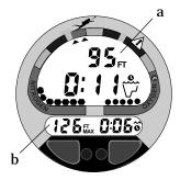
Fig. 7 - Depth Displays (No Decompression Dive)
