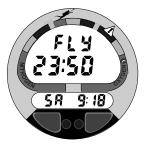
Fig. 43 - Desaturation Time (less than 9:59)
