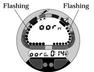
Fig. 63 - Out of Range (depth > 330 ft/99.5 m)
