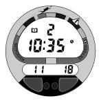
Fig. 46 - Log Mode (first screen - date/time)
