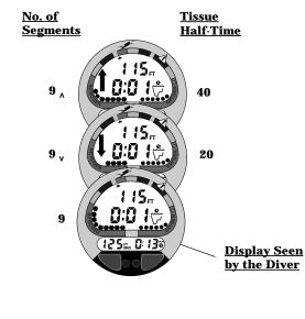
Fig. 75 - Tissue Compartment Control Hand-Over
