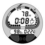
Fig. 67 - High Oxygen Accumulation (warning)
