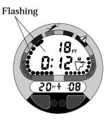
Fig. 57 - Delayed Violation (above ceiling > 5 min)
