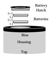
Fig. 72 - Installing Batteries
