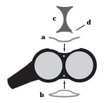
• Grasp the dual gauge unit with your right hand and push it into (toward the left) the boot feeding the hose fitting into the handle of the boot.
