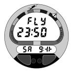
Fig. 44 - Desaturation Time (greater than 9:59)
