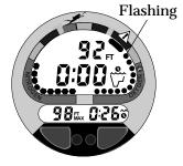
Fig. 68 - High Oxygen Accumulation (alarm)
