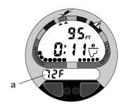
Fig. 34 - Temperature (underwater)
