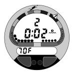
Fig. 38 - Surface Mode (less than 10 min.)
